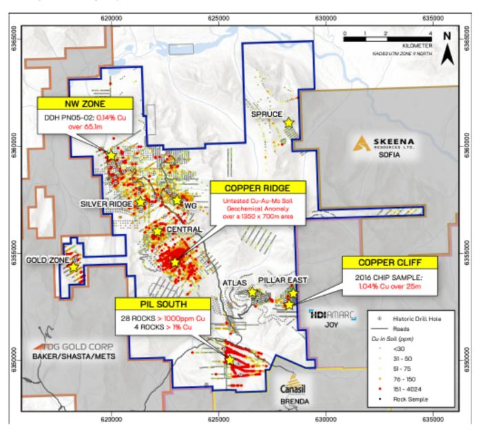
The exploration program will focus on detailed geological and alteration studies, in addition to IP geophysics to develop drill targets. Permitting for future drilling has been submitted to the Ministry of Mines & Energy and Low Carbon Innovation. Follow-up mapping and sampling is also planned at the Copper Cliff target which hosts a 25m continuous talus sample that assayed 1.04% Cu. Other targets will be investigated depending on time and budget.
