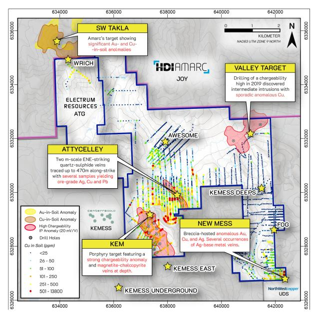
The exploration program will include geological and alteration mapping and sampling to outline the extent of the Attycelley veins and their relation to the large surrounding soil anomaly, and high chargeability IP anomaly. The Attycelley hosts several high-grade samples with values as high as 240.6g/t Ag, 9.1% Pb, 5.5% Zn, 1.8% Cu and 0.66g/t Au.
